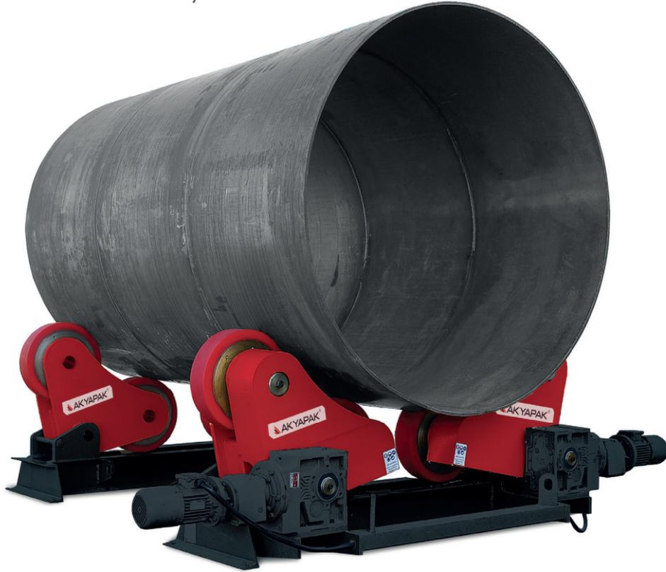
The self-aligning rotator is an ideal solution when diameter of the rotated workpiece is variable. The rotators are used for rotating tanks, pressure vessels, wind tower sections, boilers, silos, fuel barrels and such circular parts. The SAR Rotators are able to adjust wide range diameters automatically. No additional time or effort is required to start rotation of the work piece.
