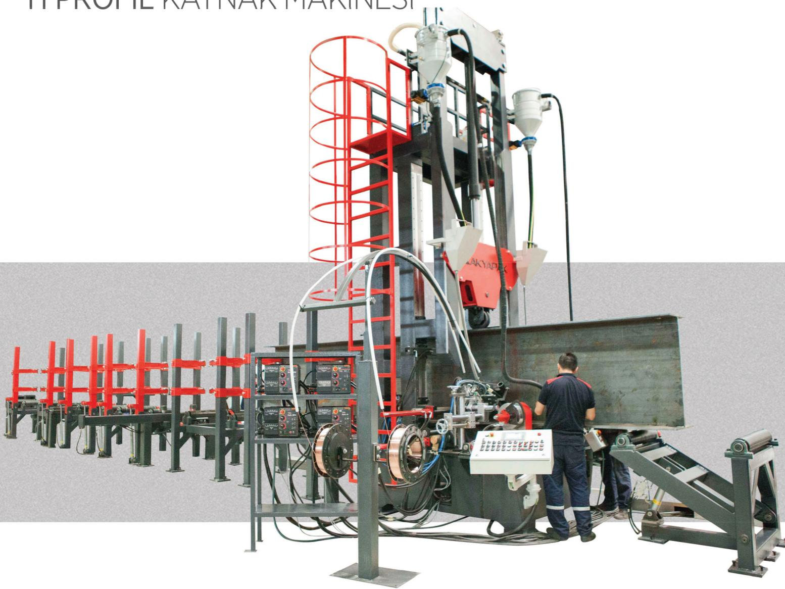
**HBW - H Profile Welding Machine** is designed to obtain required high quality special H-profiles by welding flanges and webs in different sizes centered at infeed conveyor groups again under Akyapak guarantee for fast, reliable and high quality results.
